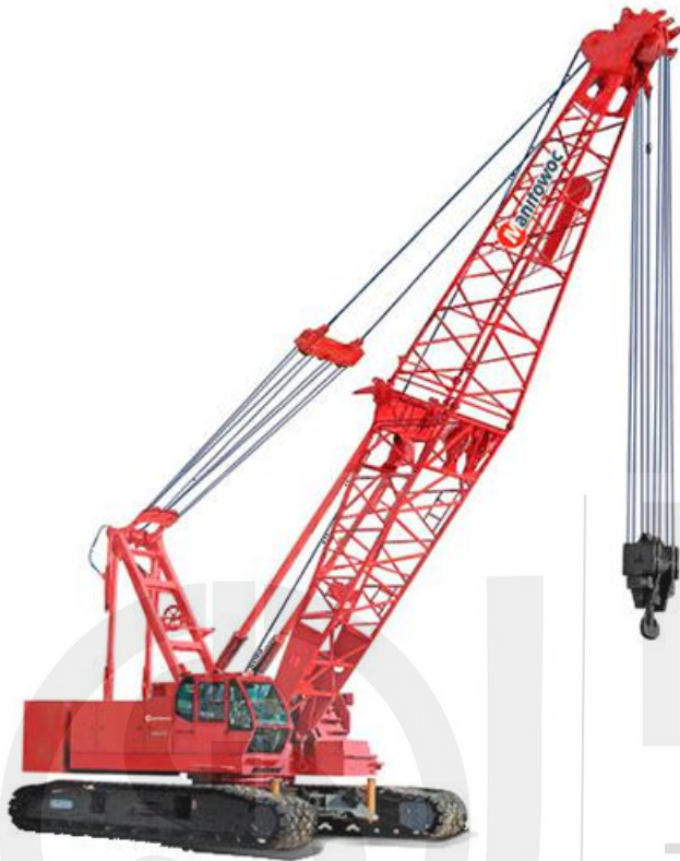
Figure 8.3: Lattice Boom Crane
