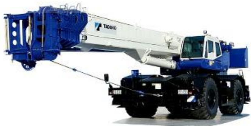
Figure 8.6: Rough Terrain Crane
