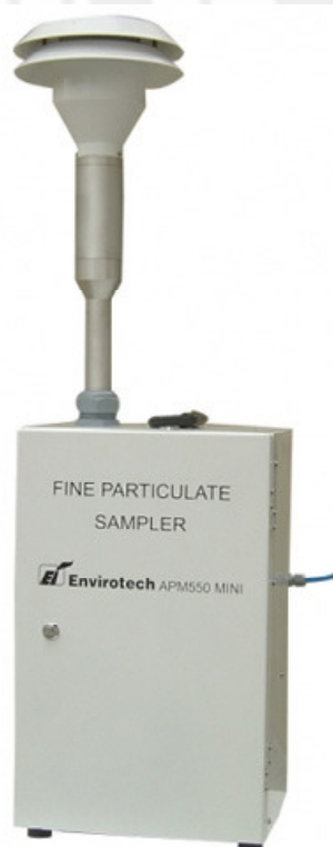
Fig.1 : PM10/PM 2.5 sampler of Envirotech, India
