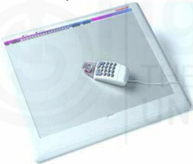
Fig. 7.3: Digitising table and puck (source: http://proceedings.esri.com/library/userconf/proc01/professional/papers/pap894/p894.html )
