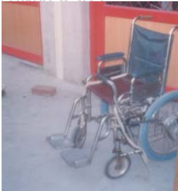
Fig. 14 : A chair with a lever fixed to the left wheel which allows the person to operate it using only the left hand.
