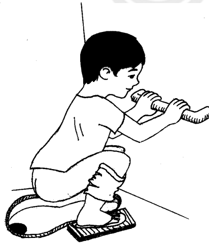
Fig. 7: Bars inside the toilet help the child to maintain balance while squatting
