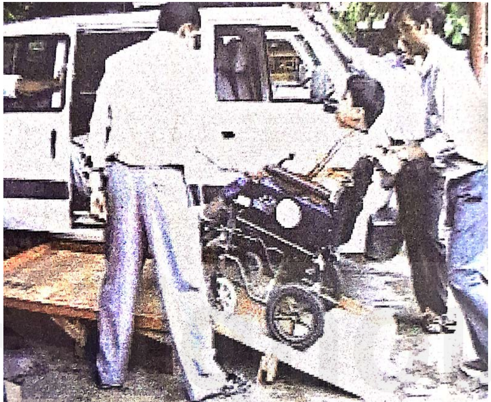
Fig. 5: Using a portable ramp to get the wheelchair at a level which makes it easier for the child to be transferred inside the van
