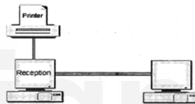
Fig 10.1 : A small LAN comprising a network between Doctor and Nurse's Station. A single printer is shared by both the computers
