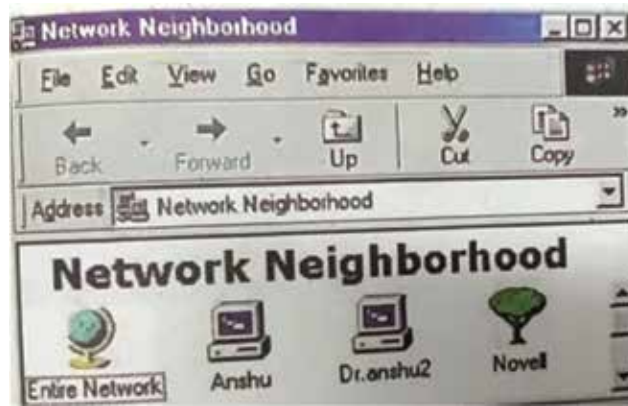
Fig. 10.7: Use of entire network lists all computers of different work group on the network
